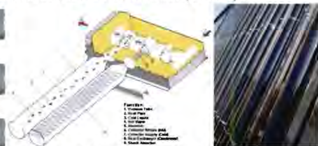
Figure 119: Evacuated tube solar water heaters - components
