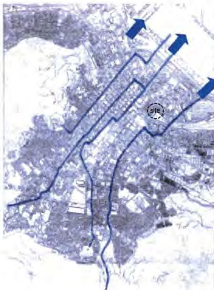
Figure 99 & 100: Clean stormwater from Table Mountain channeled into the Atlantic Ocean. It is proposed that one of these channels are used for the provision of water for the bathhouse.
