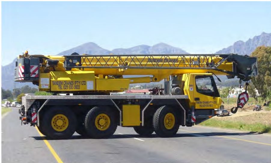
Figure 6.14: 3-axles Mobile crane
