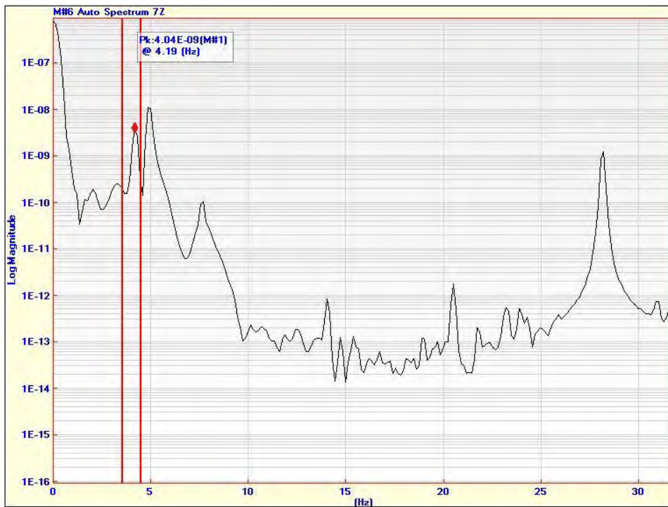
Figure 7.5: Motion of mobile crane on a plank
