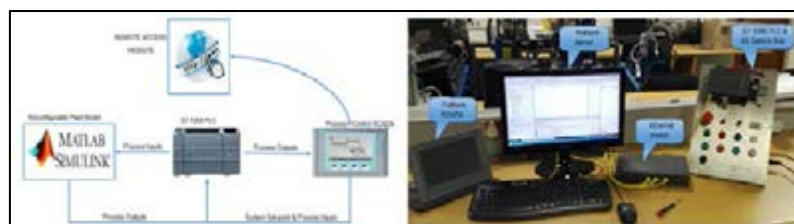
Figure 6: Online process control simulation platform integrated with real industrial hardware components
