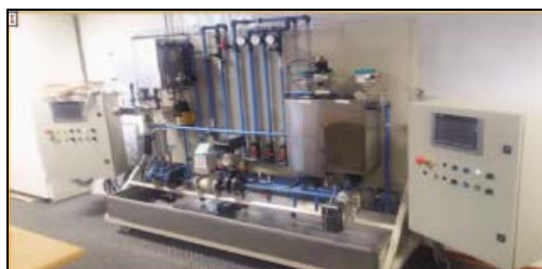
Figure 1: Multi-Disciplinary process control system
