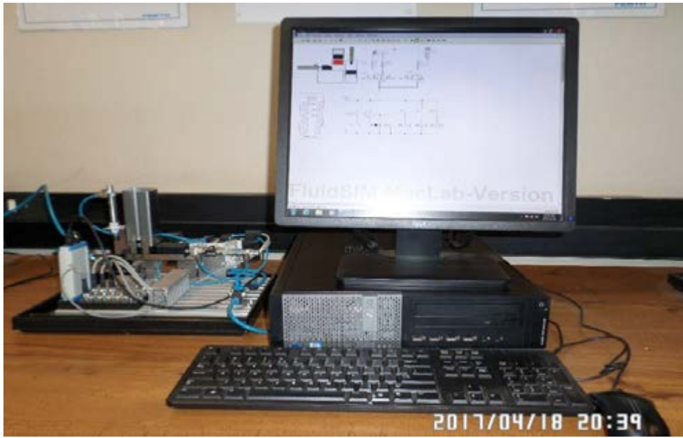
Figure 4. Festo Pick and Place equipment connected to a PC
