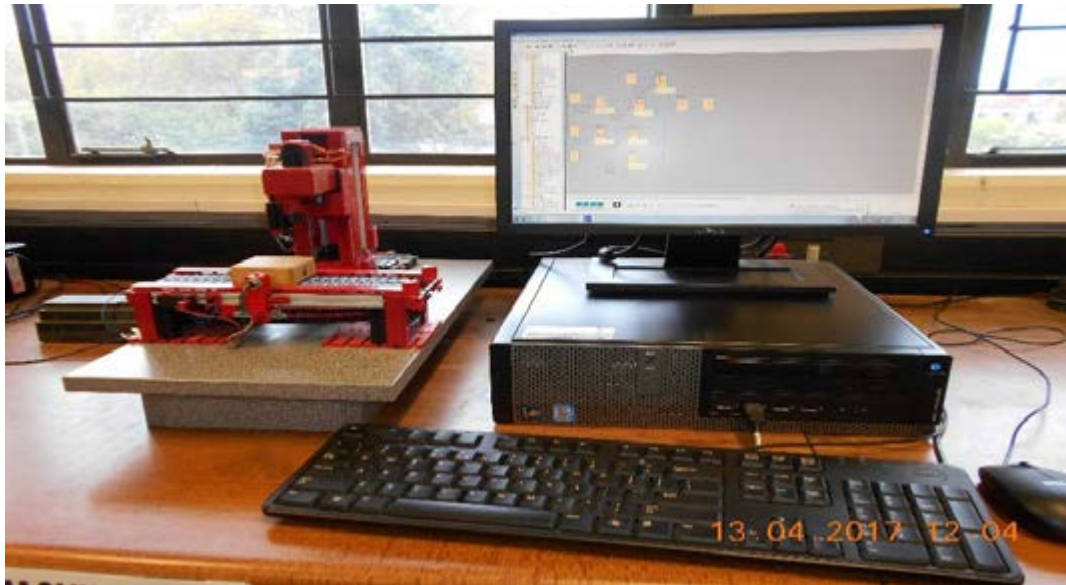
Figure 2. Conveyor belt with a machine tool attached to a PC
