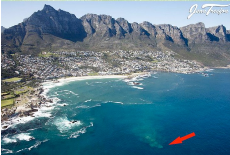
Figure 7: Sewage in Camps Bay making its way to the surface (Tresfon, 2015).
