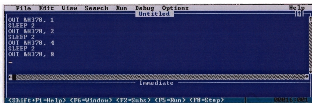
Figure 13 – Illustration of multiple lines of computer code separated by ‘pause’ statements
