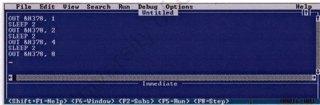
Code to step the lights sequentially
