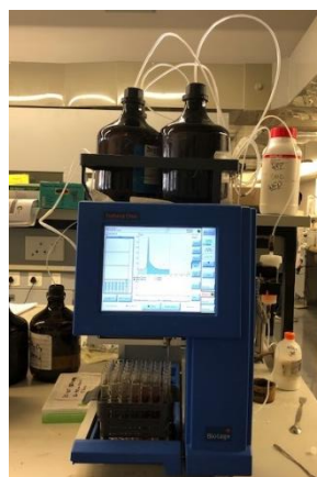
Figure 3.5 Biotage Isolera One system used for column chromatography
