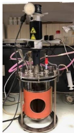
Figure 3.1 New Brunswick Scientific BioFlo 110 modular benchtop fermentor system used for 5 L working volume cultivation of P. purpurogenum . The reactor is shown, with agitator motor, pH and dO 2 probes and heating jacket visible.
