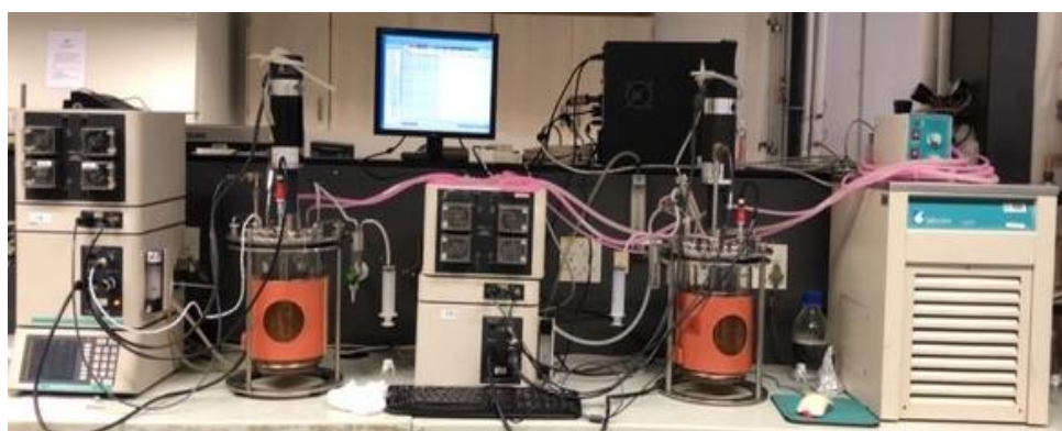
Figure 3.2 Duplicate New Brunswick Scientific BioFlo 110 reactors, with associated PCUs and common data logging and coolant circulation systems.
