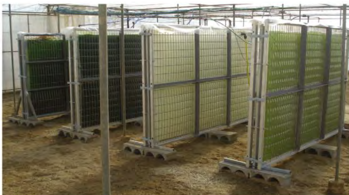
Figure 2. 9: Photograph of “green wall panel” photobioreactors (GWP) at the University of Almeria in Spain (Lehr and Posten, 2009)
