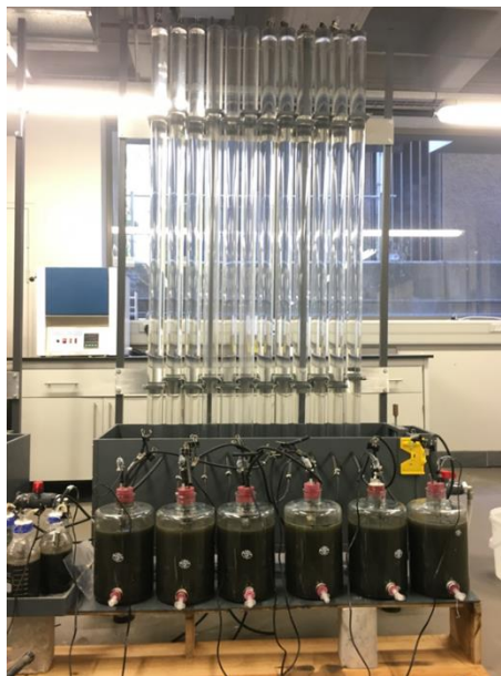
Figure 3-4: Experimental set-up for an ABMP test (Maake & Ikumi, 2021)
