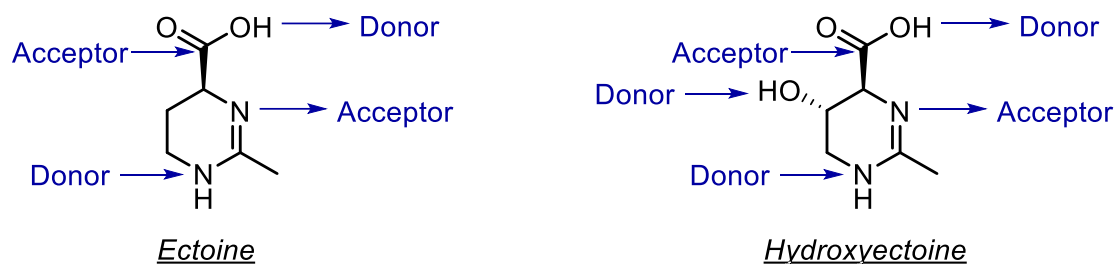
Figure 62: The chemical structure of ectoine and hydroxyectoine, compatible solutes utilised in this study, together with their H-bonding profile.
