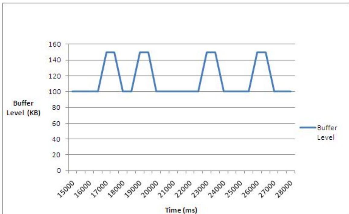
Figure 5.13: Proxy buffer usage during hard handoff
