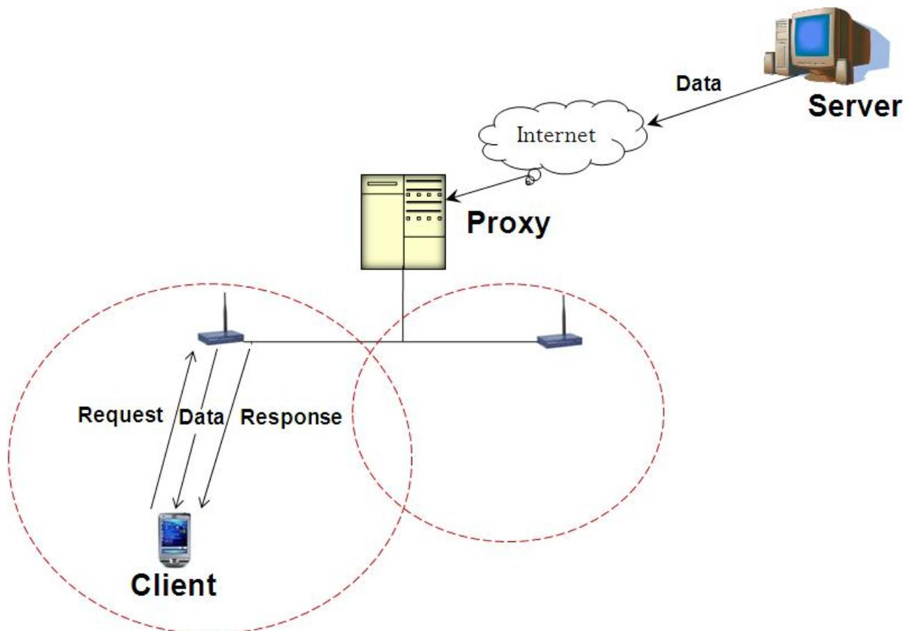
Figure 4.1: High Level Middleware Components
