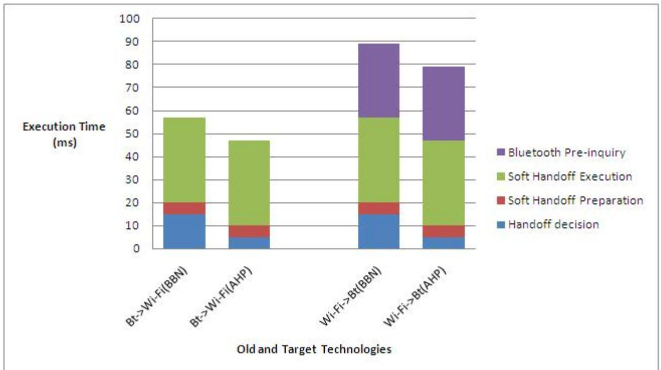
Figure 5.12: Overall Soft Handoff Execution Time between Bluetooth and Wi-Fi
