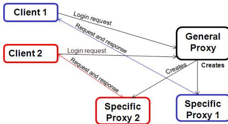
Figure 4.2: Proxy and client interaction
