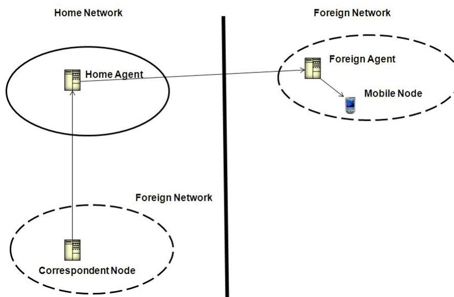
Figure 2.6: Components of MobileIP
