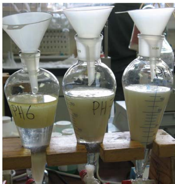
Figure 4-20 Photographs showing the stable emulsions formed in the organic phases in separating funnels from the pH dependence test work for Alamine 336. Stripping was conducted at pH values 6, 7 and 8.
