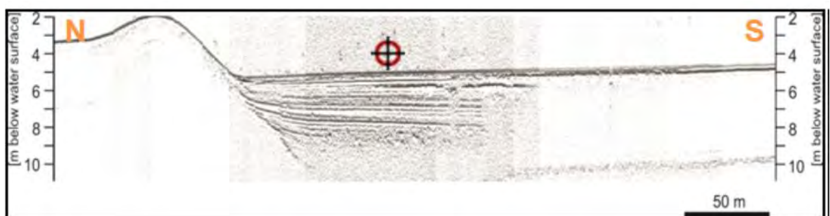
Figure 4.6 The seismic profile for Eilandvlei indicating the location of the EV1.11 core (Courtesy Kasper 2013; Kirsten 2014)
