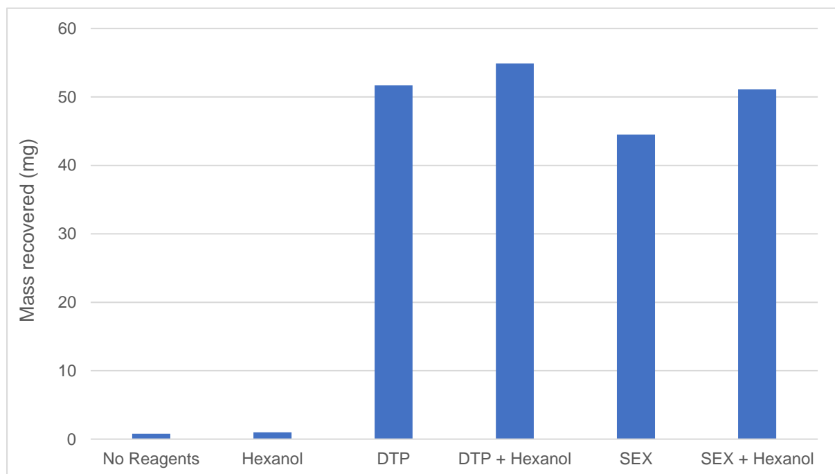
Figure 4.17: Mass recovery of chalcocite (pH9), under various reagent environments. Collectors are dosed at 50% monolayer coverage and the frother is dosed so that the concentration is just above the CCC. (Contact time = 50 ms)
