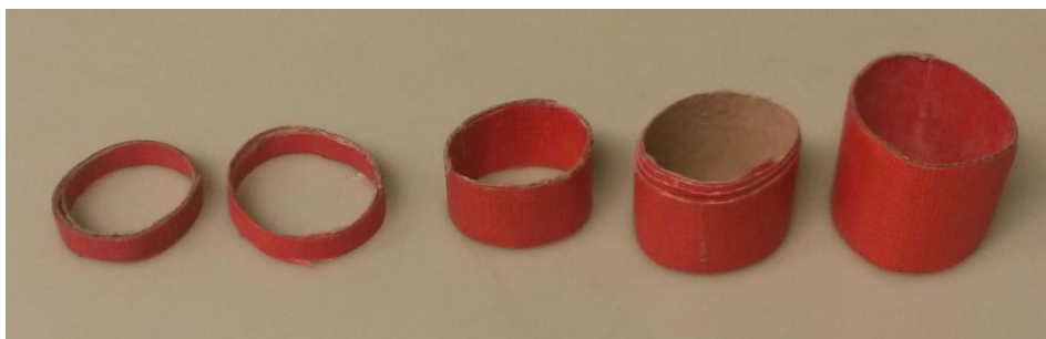
Figure 3.13: The cylindrical rings used to contain particles in a bed for breakage tests, arranged in increasing number of layers contained in the bed
