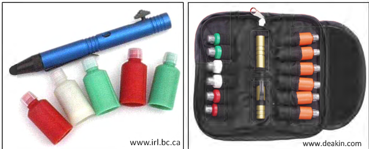
Figure 2.5. Examples of bear banger cartridges and pen launchers. The cartridge bases are fitted to the broad end of the launcher. When the launcher's trigger is released, it initiates a primer (initial 'pop' sound) in the cartridge as well as a delay pellet. The primer causes the pellet to launch, while oxidation of the flashpowder in the delay pellet results in a loud bang a few seconds later (and 20-30m from the ground if aimed correctly).
