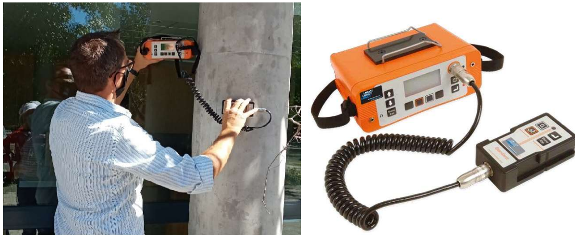
Figure 4-9: Use of covermeter for cover depth and measurement of rebar location and size [92]
