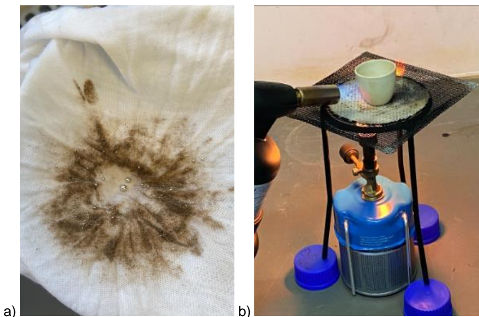
Figure 37: a) no visible amalgam ball recovered b) burning of small particles potentially being amalgam particles
