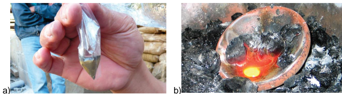
Figure 8: a) borax mixed with concentrate b) Melted concentrate (Appel and Na-Oy, 2012)
