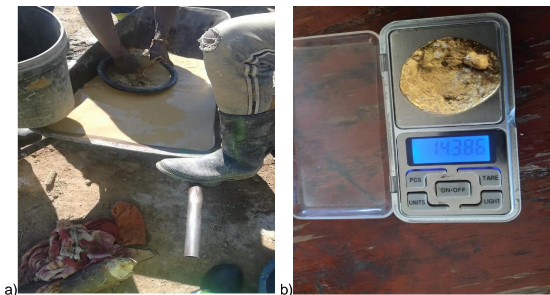
Figure 79: a) concentrate panned with mercury b) gold sponge obtained after amalgam burning
