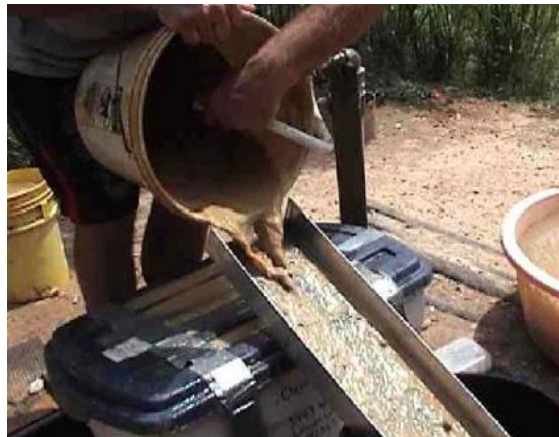
Figure 6: Cleangold sluice (Vieira, 2006)
