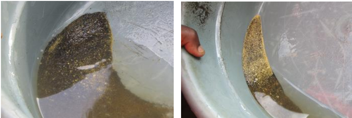
Figure 12: a) Centrifuge discharge (left), b) 89-93% gold concentrate post magnetic separation (right) (Drace et al., 2012)
