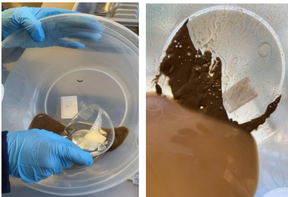
Figure 36: Mixing of mercury and ore concentrate
