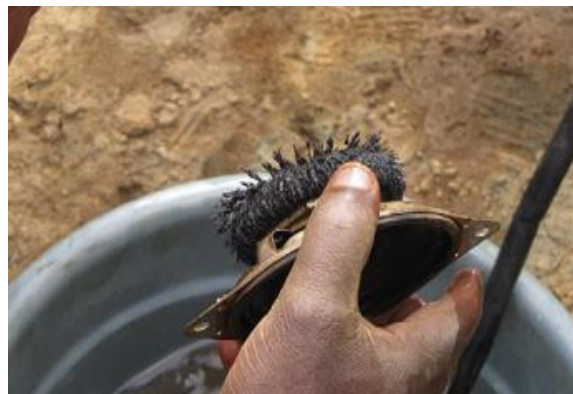
Figure 13: Magnets from radio speaker used for magnetite removal (Drace et al., 2012)
