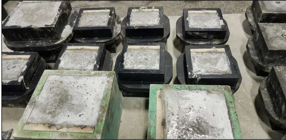
Figure 3-2: Composite specimens with the concrete cast against the fibre cement boards in the cubic moulds.
