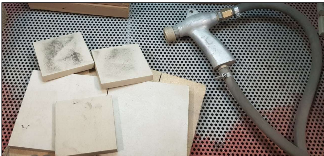
Figure 3-1: Sandblasting machine used to improve fibre cement boards surface roughness
