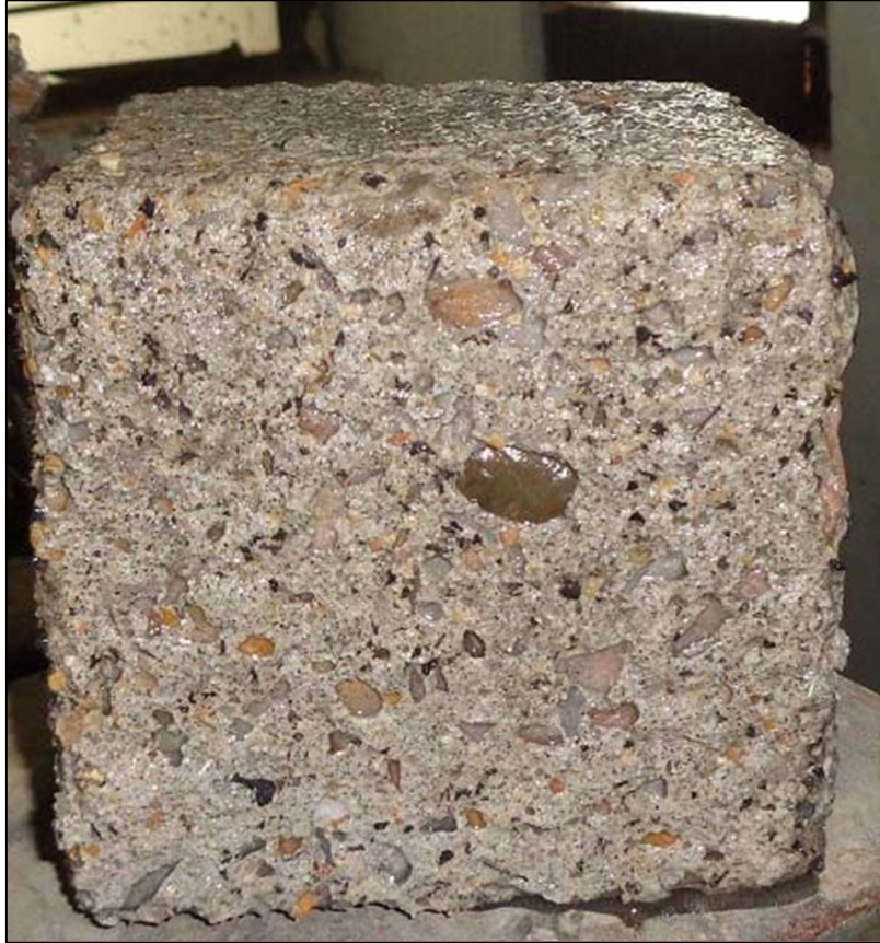
Figure 2-6: Concrete cube exposed to sulphuric acid for 84 days (Kumar & Gupta, 2015)
