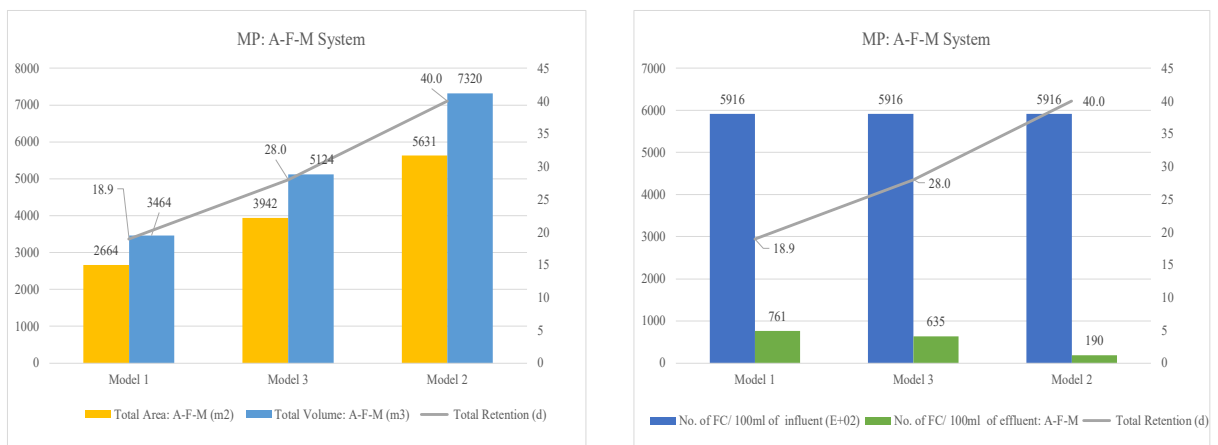
Figure 4.10: The required total area, volume, retention time, and the influent and effluent FC of the MP for the A-F-M system for Scenario 1.
