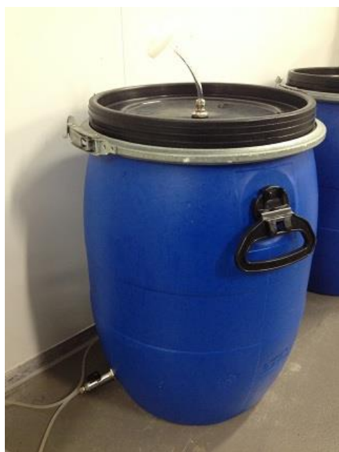
Figure 3-3: Feed drums used for after start-up of the first experiment
