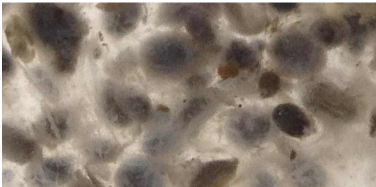
Figure 5-1: Sludge granules after being underfed for four months
