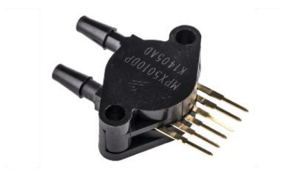
Figure 16: NXP MPX5010DP pressure sensor
