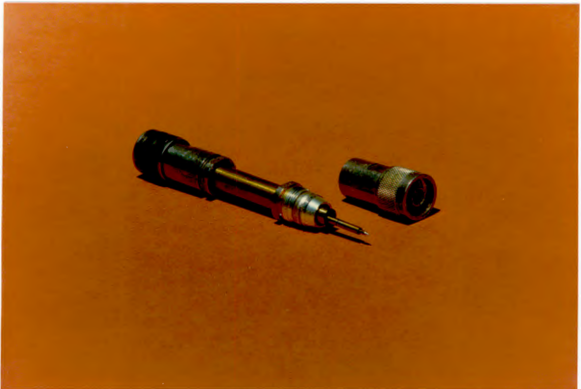
Figure 7.8. Coaxial Test Structure
