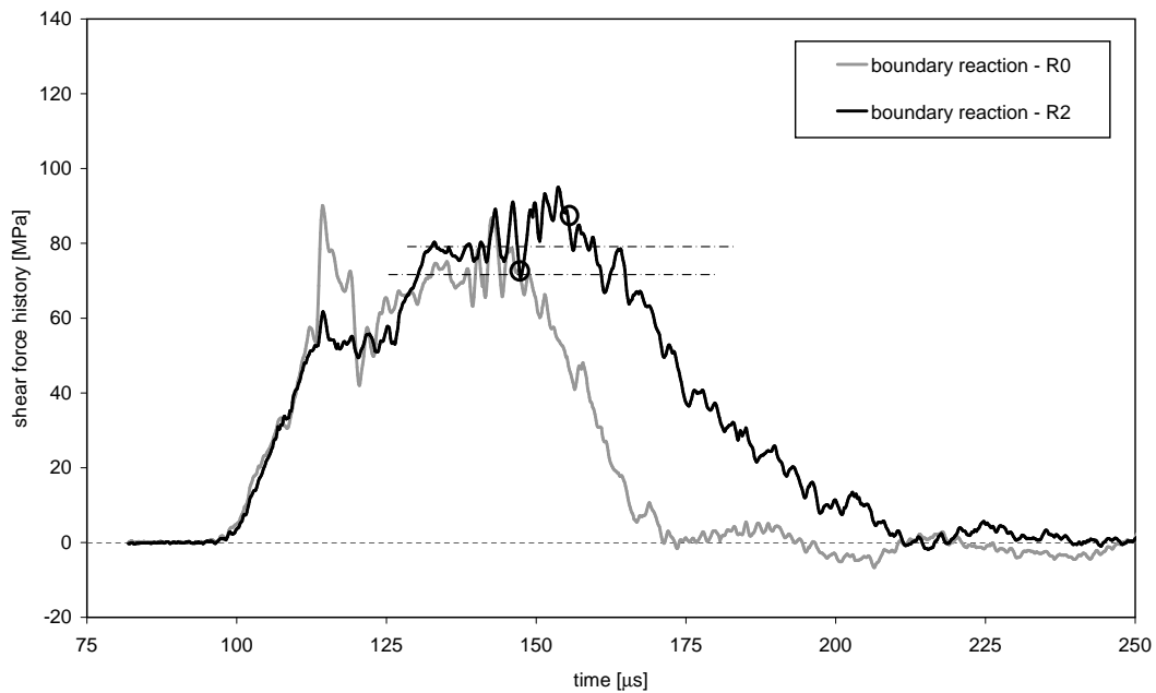
Figure 6.33: Comparison of the Mode III PCCS shear force history estimates shown in Figure 6.32 for R0 and R2 central support boundaries.
