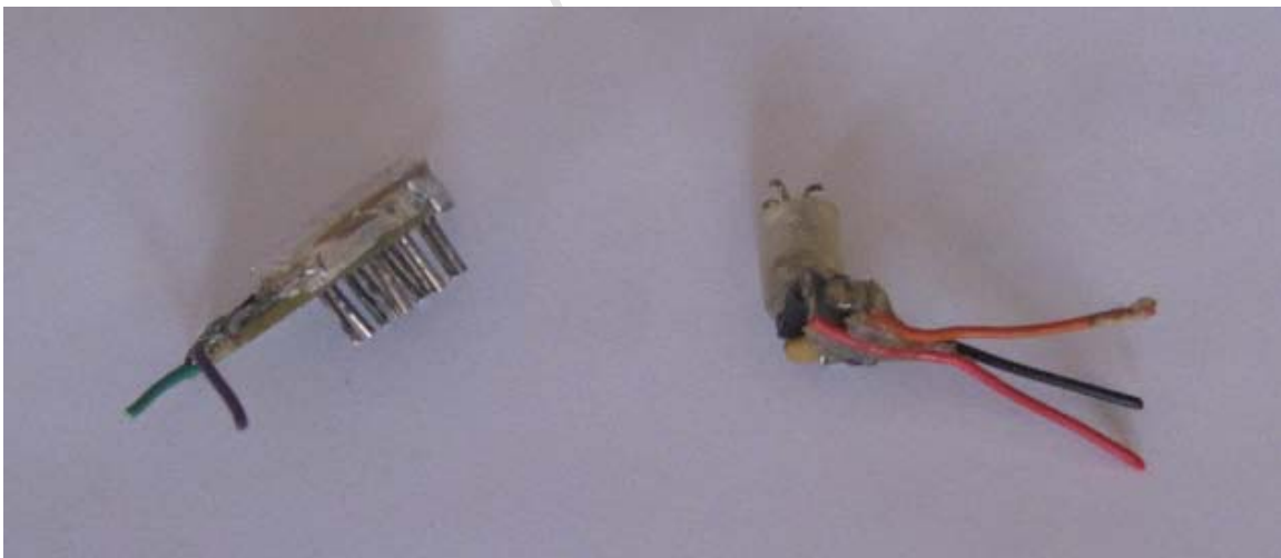
Figure A3. An electrode with spikes (left) allows the scalp to be reached through hair. The active electrode (right) has wires for power and the signal.
