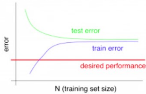
Figure B-17: Error vs training set size curves for a high bias model [27]
