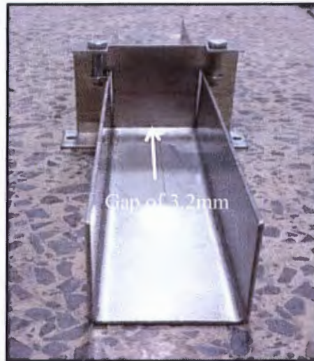
Figure 3.14: The applicator used to apply a constant epoxy adhesive thickness
