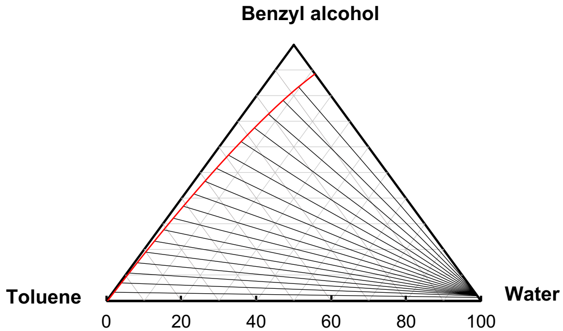
Figure B-4.3: Ternary phase diagram of the liquid-phase in the system benzyl alcohol + water + toluene at 80°C with tie-lines.
