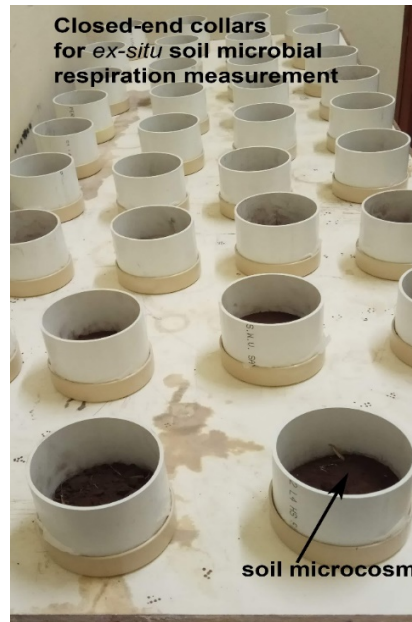
Figure 5.2: Illustration of the ex-situ soil microbial respiration measurement collars closed at the bottom end.
