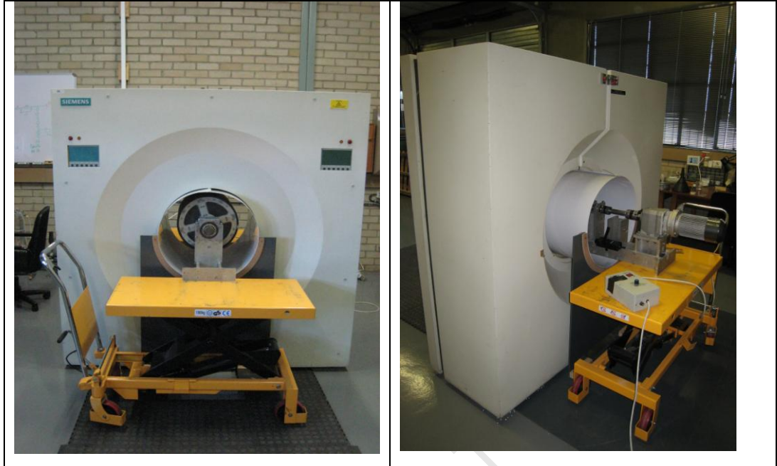
Fig 22: The experimental mill in the ECAT EXERT3D camera system at PEPT Cape Town.
