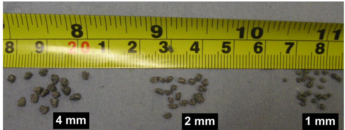
Fig 17: Illustration of the tracer particles employed in the PEPT experimental work at UB.
