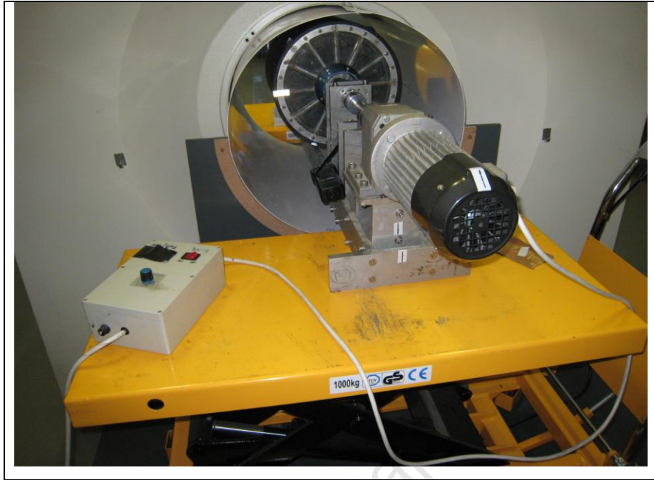
Fig 24: Setting the mill speed with an optical switch at PEPT Cape Town.
