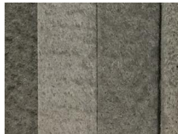
Figure 2-8: Typical non-woven geotextile with varying thickness and pigmentation
