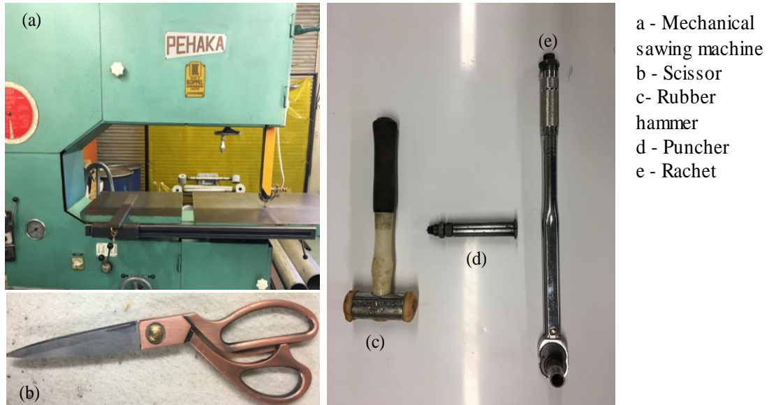
Figure 3-5: Accessories used in test sample preparation
