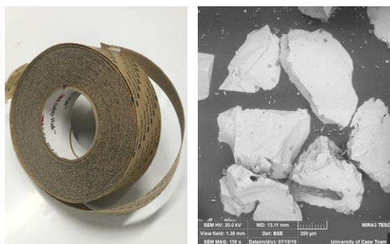
Figure 3-11: (a) 3M sandpaper roll (b) 150 x magnification of sandpaper SEM
