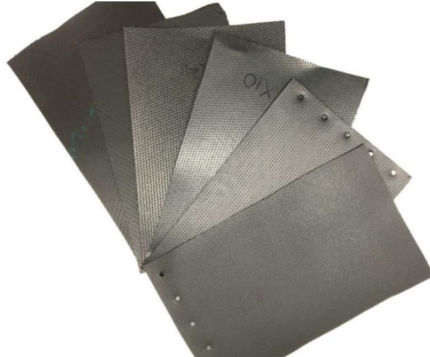
Figure 2-11: Calendered geomembrane textured products
