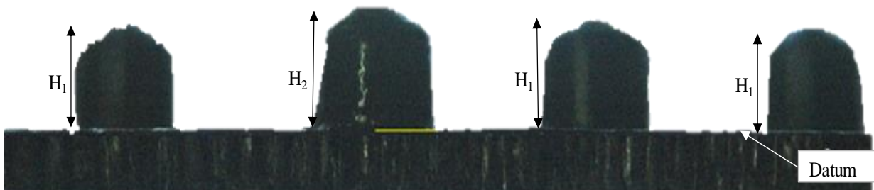
Figure 3-7: Magnified view (6.3x) of textured geomembrane asperity
