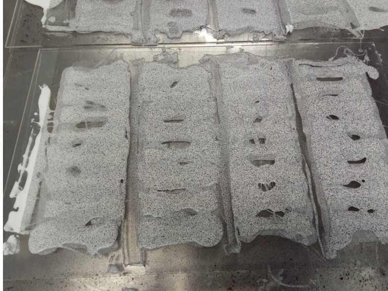
Figure 4.3 Photograph of uniaxial Dragon Skin 10 specimens in their mould after being speckled with an air brush
