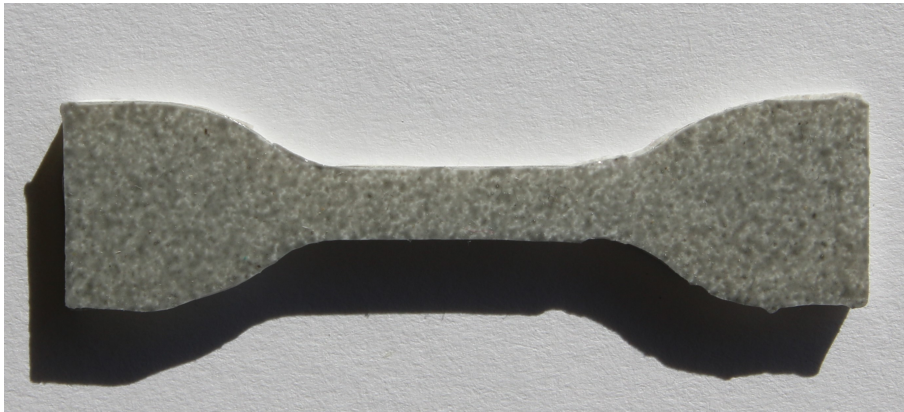
Figure 4.1 Photograph of a failed uniaxial Dragon Skin 10 specimen which was speckled using an airbrush
