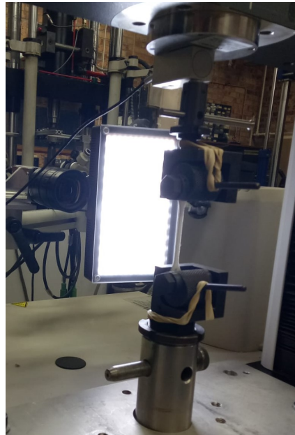
Figure 5.6 Specimen under tension in Instron machine
