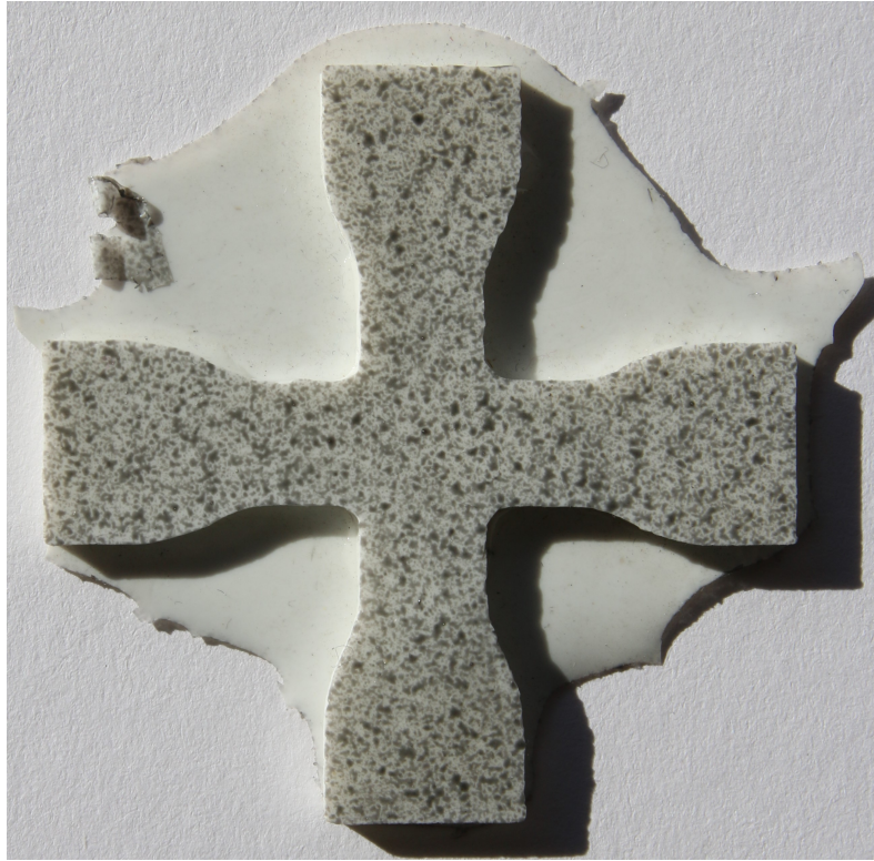
Figure 4.2 Photograph of a successful biaxial Dragon Skin 10 specimen after being speckled with an air brush, before having the excess silicone trimmed
