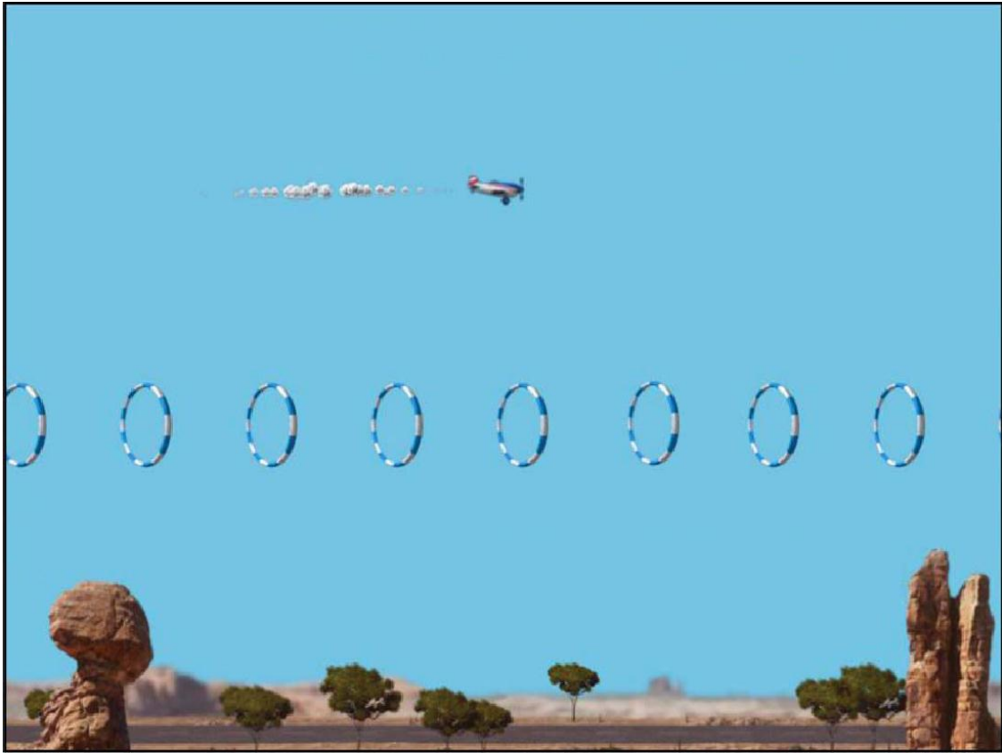
Figure 4.1: The position of the moving object (plane) reflects the superior/inferior motion of the diaphragm. Expiration decreases the altitude of the object and inspiration increases it. The loops represent the desired end-expiratory position.
