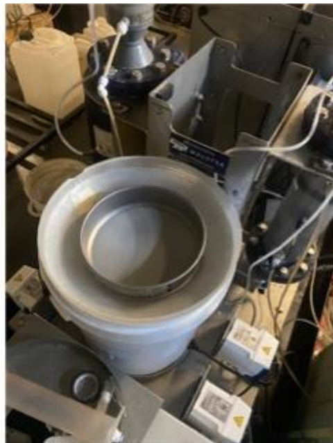
Figure 3.6 | Adding PT DWW to Feed tank
