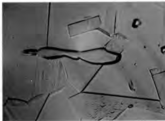
Figure 31 Microstructure of the 316NG material after sensitizing at 650°C for 24 hours. Etched in 10% oxalic acid solution in accordance with ASTM 262 – A.
