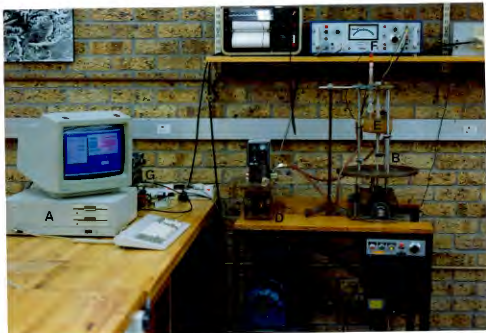
Figure 18 Photograph of the slow strain rate rig used in this investigation. A. Computer used for data capture; B. Load frame; C. electric motor; D. Water bath; E. Test cell; F. Potentiostat; G. Control electronics.
