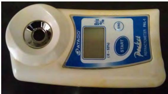
Figure 32: Refractometer used for measuring frother concentration
