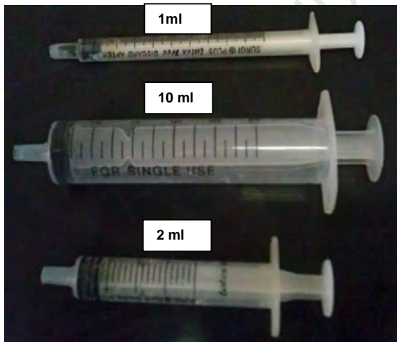
Figure 34: Graduated syringes used for dilution of the frother sample and to make up frother solutions for tests
