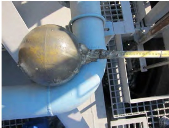
Figure 27: Measuring the froth depth
