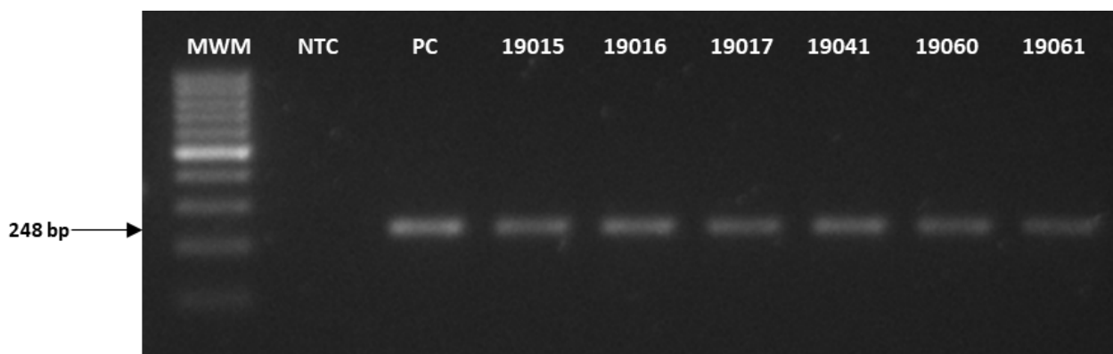
Figure 3.5: A representative gene for PCR amplification. The image indicates PCR fragments run at 100V for 1 hour on a 1.5% agarose gel for PIK3CA exon 9. In the first lane is the molecular weight marker (MWM), the GeneRuler™ 100bp Ladder (Thermo Fisher Scientific), the second lane is the non-template control (NTC), and the third lane is the positive control (PC). The following lanes are individual samples. The amplicon was 248bp. The other genes were done the same way (Appendix I); the amplicon sizes for them were as follows: TP53 exon 4: 353 bp, PIK3CA exon 20: 231 bp, PTEN exon 5: 236 bp, EGFR exon 19: 399 bp and EGFR exon 20:374 bp.
