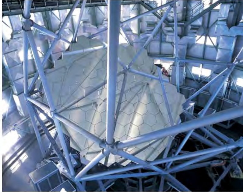
Figure 3.5: The SALT primary mirror array which consists of 91 hexagonal 1-m segments, with an accuracy of 15.7 nm RMS and a master sphere radius of curvature of 26.165m. Adopted from figure 1 of Buckley et al. (2006a).
