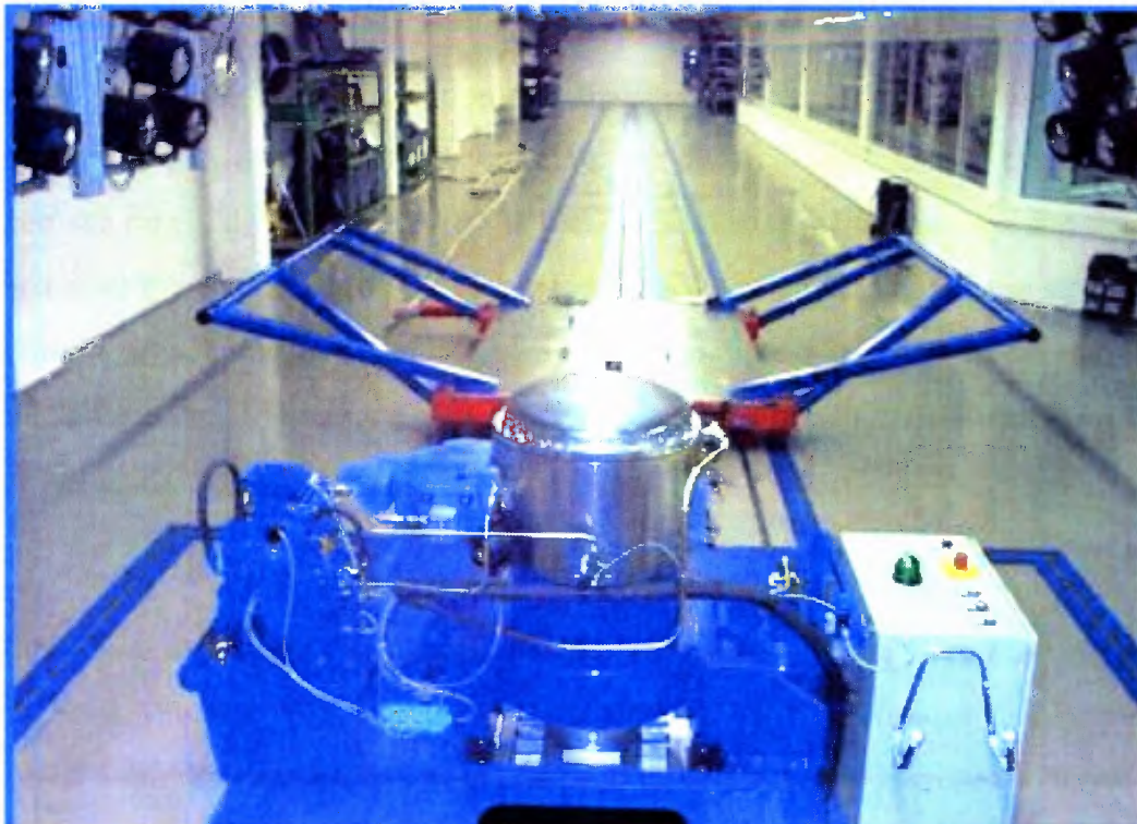
Figure 2-8: Picture of a MESSRING sled tester system taken from the deceleration end [9]
