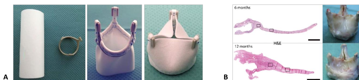
Figure 3.4: Approach to fabricating a tissue engineered heart valve from an electrospun polymer tube. A) Valve manufacturing process. B) H&E analysis of leaflet explants showing variable interleaflet thickness (adapted from Kluin et al. 149 )
