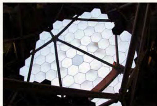
Figure 3: Image taken from: (Crause, 2010): Learning from the tessellated mirrored structure of S.A.L.T
