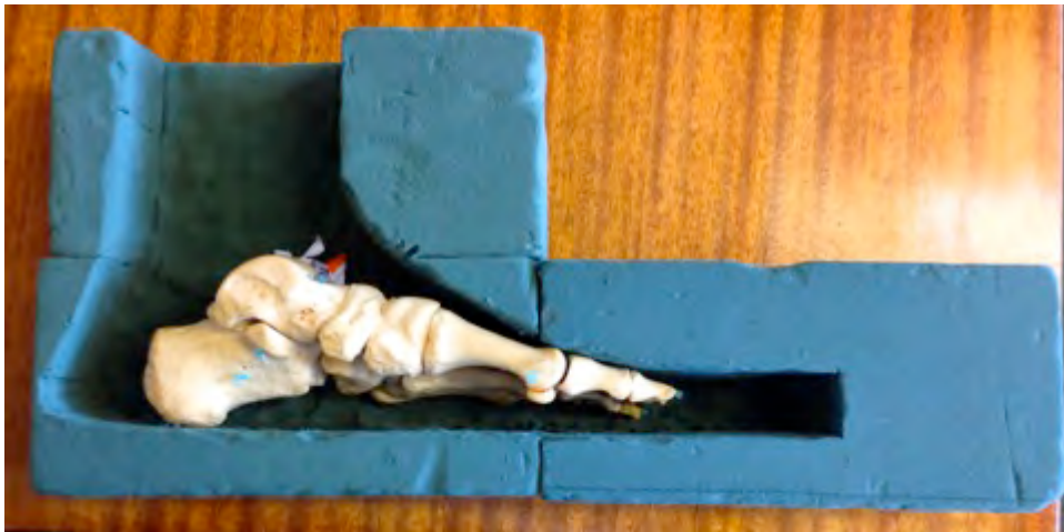
Figure 11 Photograph showing mould after foot shape was cut out.
