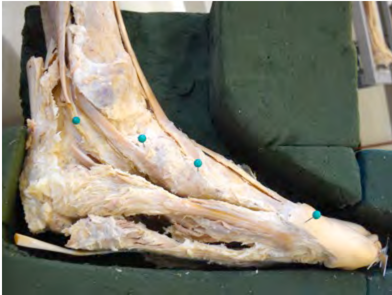
Figure 12 Photograph showing implementation of foot mould with cadaver foot in place and pins placed on bony landmarks.
