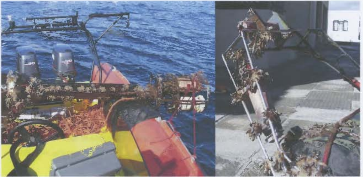
Figure 2-3 Photographs of BOB removed from mooring for monthly servicing, illustrating levels of bio-fouling on buoy and instruments. The SCUBA and radiance sensor can be seen wrapped in copper sheet which helps to reduce local fouling (left)
