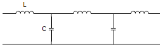
Figure 2.6: The absence of R and G shows an ideal lossless transmission line.
