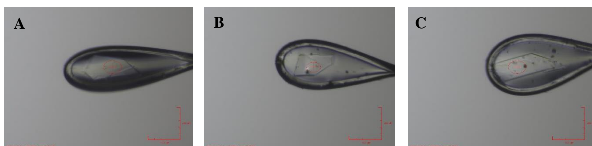
Figure 3.9: rHDP crystals mounted on a cryoloop under the Diamond Light Source Viewer.
