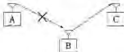
Figure 5.6: Transmission A to B collides with transmission B to C: transmission B to C succeeds, transmission A to B fails
