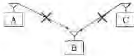
Figure 5.5: Transmission A to B collides with transmission C to B: both transmissions fail
