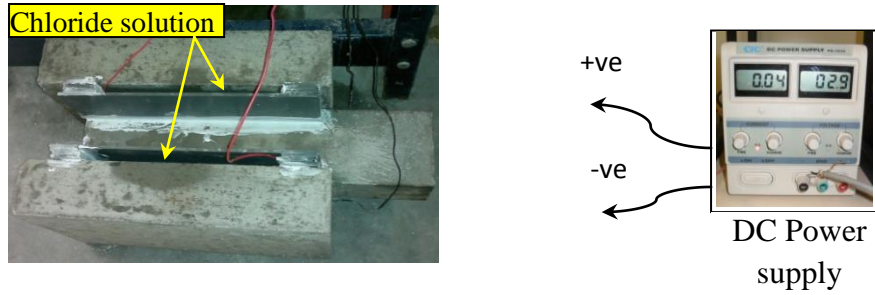
Figure 4.7: Set up for accelerating corrosion on shear connectors in push-off specimens
