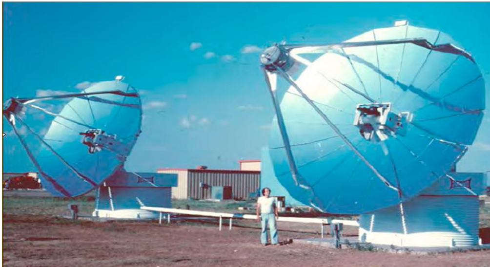
Fig.2. 1: The Ominium-G Parabolic Dish collector [14]
