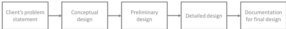
Figure A 1 "Normal 'linear' models for design process" by Dym et al. (2009).
