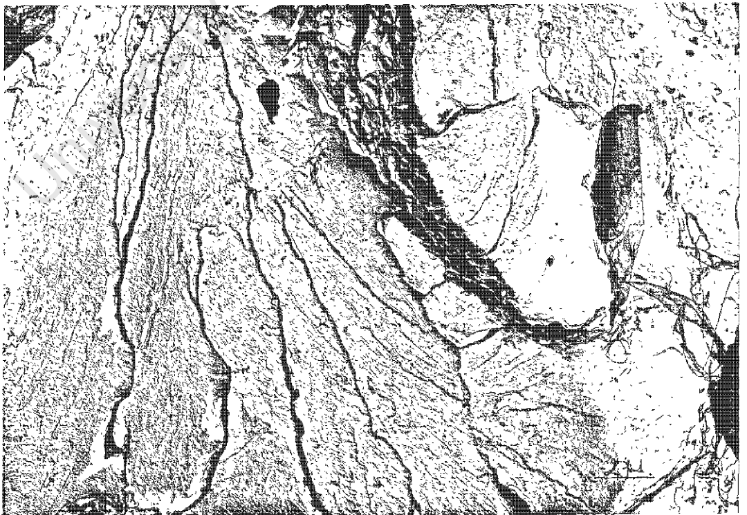
Figs.1-2 Cleavage fracture in low carbon steel showing area of dimple rupture (microvoid coalescence) near
