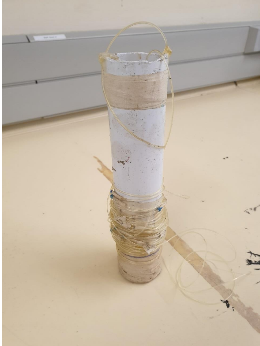
Figure 8 Improvised depth meter used to measure the borehole water level
